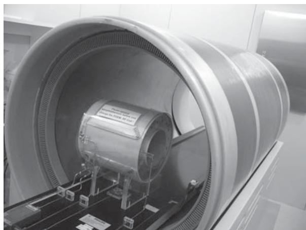
Figure 1. Photograph of an OMRI scanner including the main magnet and OMRI composite-resonator.
